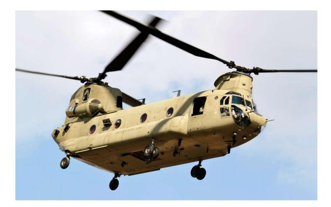
**The Boeing CH-47 Chinook** is an American twin-engined, tandem rotor, heavy-lift helicopter developed by American rotorcraft company Vertol and manufactured by Boeing Vertol
