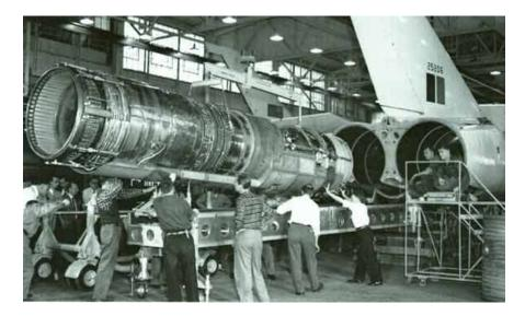
The Orenda PS-13 Iroquois engines, which the Avro Arrow were equipped with, were absolutely the best and most powerful engines on the continent. - (best weight-to-thrust ratio, most efficient fuel consumption)
